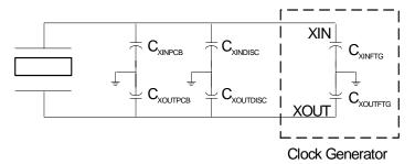
As an example and using this formula for this data sheet's device, a design that has no discrete loading capacitors ( $C_{DISC}$ ) and each of the crystal device PCB traces has a capacitance ( $C_{PCB}$ ) to ground of 4 pF (typical value) would calculate as follows.
