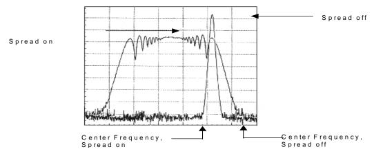
Figure 1. Spread Spectrum
